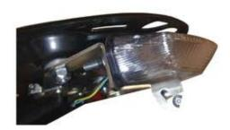
Install the tail light using the bracket and mount it under the Barracuda saddle specific frame using the appropriate special connection and the supplied screws.
