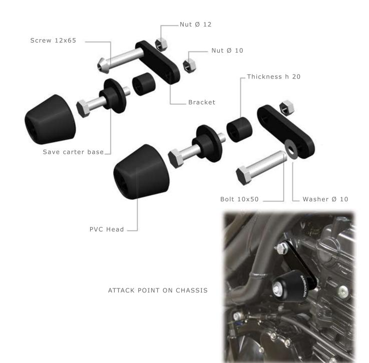
SEARCH AND FIND THE FIXING POINT ON THE MOTORBIKE BEFORE START TO MOUNTAIN, USE THE SPE-CIFIC THICKNESS AND BOLTS LIKE DESCRIBED IN THE PICTURE (SO YOU CAN GET THE RIGHT PROMI-NENCE FROM THE MOTORBIKE). FIX THE PVC HEAD AFTER FIXED AND TIGHTEN ALL THE KIT ONLY
