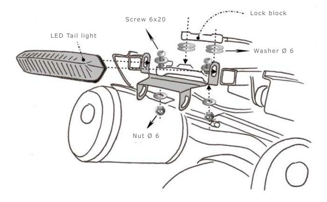
REMOVE THE ORIGINAL LICENCE PLATE INCLUDING THE IRON STIRRUP UNDER THE LOCK SO SPACE THE LOCK WITH THE TWO DIAMETER 6 WASHERS (TWO FOR EACH PART).
